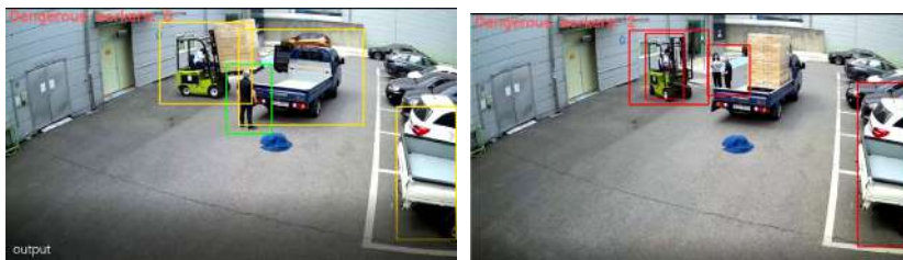
Fig. 2. Example results for non-dangerous(left) and dangerous(right) situations for moving objects
