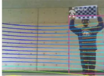
Fig. 3. Data fusion of Lidar and Camera
