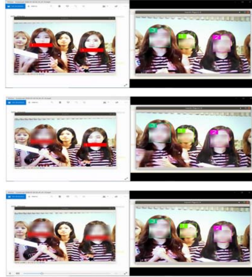
Fig. 4 Left side is the results of non-tracking blur system where a registered person is recognized as a new person and blurred. On the right side is tracking blur system where the ID is consistent in each frame.
